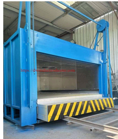
HLQ medium frequency Q&T line for steel bars, and an HLQ electric resistance bogie hearth furnace.
