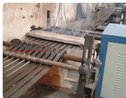
Strip: inline induction heating line.
