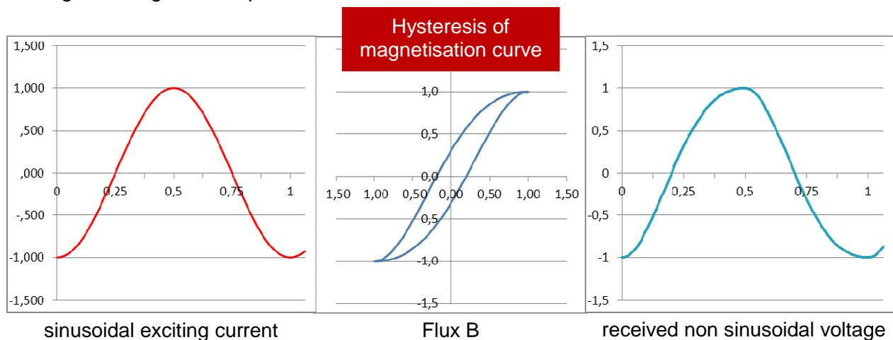
Fourier analysis of that voltage  $u$ , reveals higher frequency components of the **fundamental wave**, namely harmonics of the **3-** and **5-**times frequency. Analysis of these harmonics provides a much more precise view of the magnetic features of the test part and thus detailed information on its structure. The signals of the harmonics, however, are very small. A significant electronic effort is required to extract such small signals from the noise and to display them.
