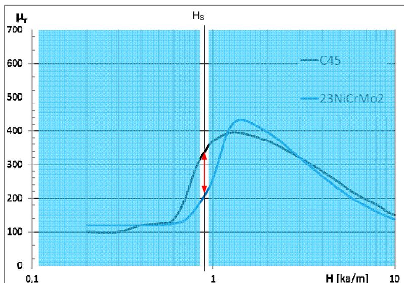
But beware: If permeability is tested with a single magnetic field strength  $H_s$ , test results may be unreliable as soon as other types of mixed parts become involved. Let us take a typical mixed part test of two kinds of steel: C45 and 23NiCrMo2. The largest difference in permeability is at  $H_s$ . This test can be done with a single frequency test instrument set up with that field strength, because this setting provides the largest difference between both.
