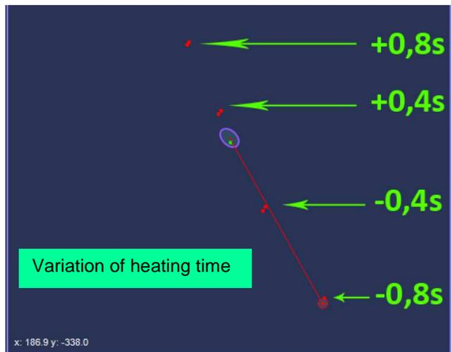
This display of the 3<sup>rd</sup> harmonic of 1.2 kHz gives a significant expansion of the eddy current signals.
