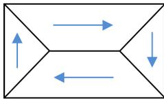
First there is formation of the domains and Bloch walls without external field  $H$ . The magnetic circle is closed within the material.
