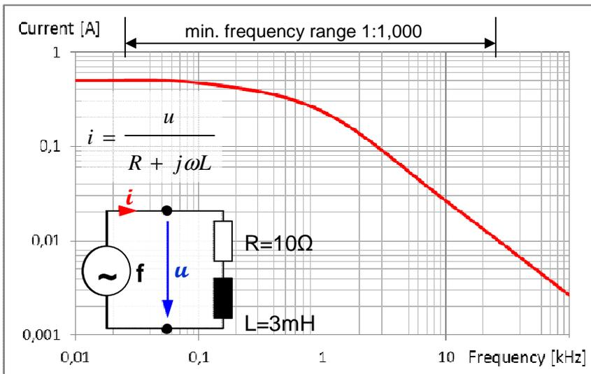
That is the "Preventive Multi Frequency Technology" (PMFT) invented by ibg which uses eight test frequencies that cover a wide area of the coil current and thus field strength. The frequency range from the lowest to the highest frequency should be at least 1:1,000 in order to vary, via the inductivity of the sender winding, the exciting current and thus the field strength in the coil.
