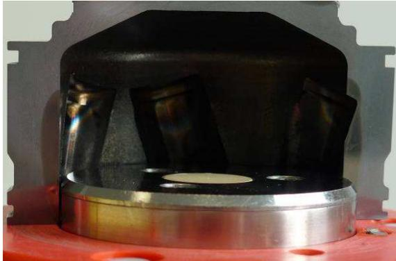
Exact insertion depth of the test coil and the coil design are decisive for a high sensitivity test against the requested hardness run out.
