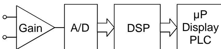
into a digital signal processor (DSP) and converted within shortest time (2 ms) to a  $2 \times 32$  bit data word. This is compared with the stored tolerance zones and a test result is given.
