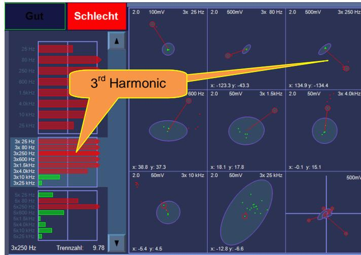
eddyvisor® (digital), NG part displayed, best separation at 3 x 250 Hz harmonic wave
