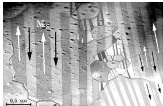
Domain structure of Fe-3%Si polycrystals with crystallites
