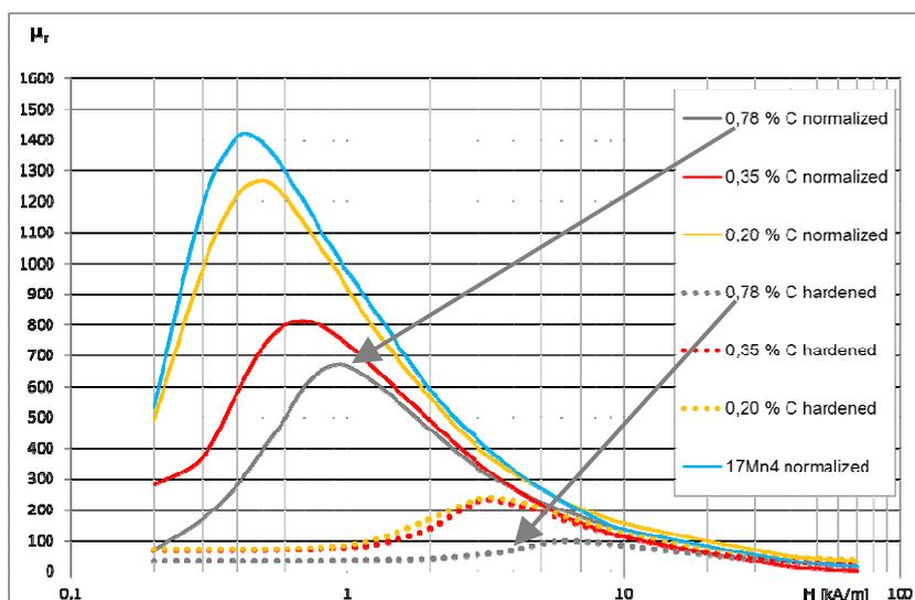
Relative permeability [ $\mu_r$ ] is strongly affected by heat treatment. The amount of carbon and other alloy elements significantly influence the size and course of the permeability curve. Generally, hardened (stressed) structures have lower permeability than soft structures (refer to graph of 0.78% C).
