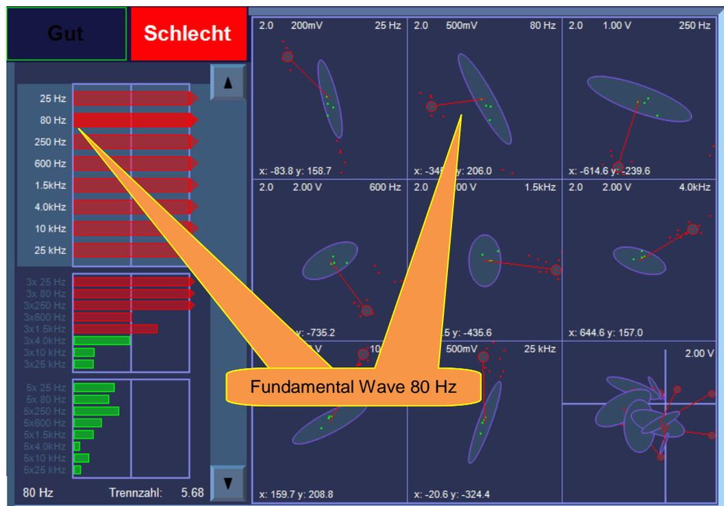
eddyvisor® (digital) in sorting mode, NG part displayed, best separation at 80 Hz fundamental wave
