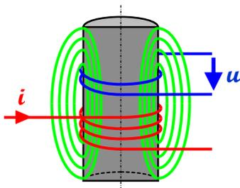
How can one get *values*? The alternating current  $i$  which flows through the red coil created a magnetic flux  $[B]$  through the test part (grey in the sketch). The size of the magnetic flux and thus the size of the voltage  $u$  induced in the blue coil is directly dependant on the electrical conductivity  $[\sigma]$  and on the magnetic "conductivity" (permeability  $[\mu_r]$ ) of the test part in the coil.
