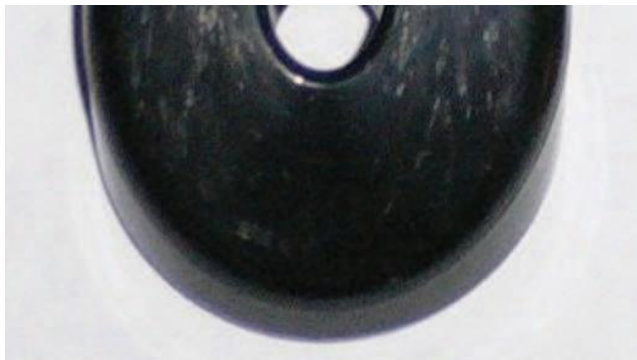
Fig. 3. Warpage and silver streaks at bottle Opener
