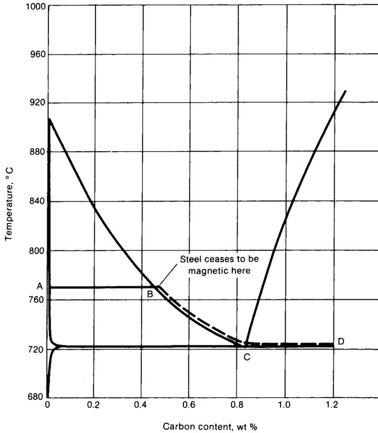
**Fig. 2.4** Curie temperature for carbon steels. Source: Ref 2
