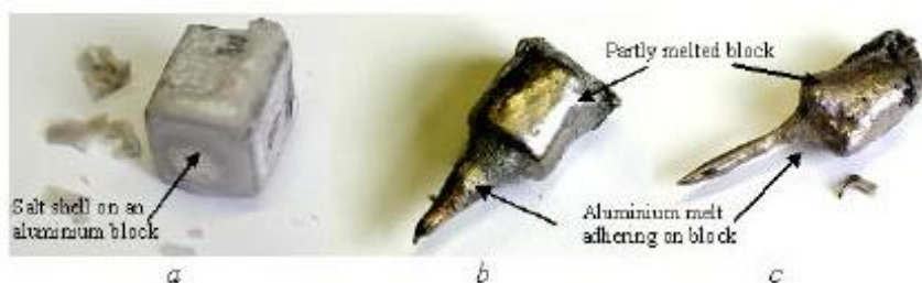
Fig. 5: scrap cube melting in molten salt and Aluminum melts
